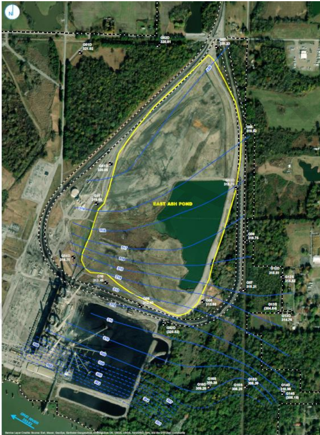
Figure 2.2 Monitoring Well Locations and Groundwater Elevation Contours for the UA. Source: Ramboll (2022).
